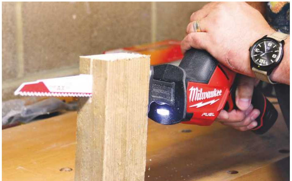
▲ Fitted with a longer blade it's more than powerful enough to rip 75mm timber
